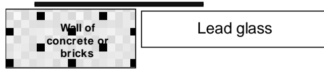
FIG. 6 SHIELDING ROUND THE EDGE OF AN OBSERVATION WINDOW
